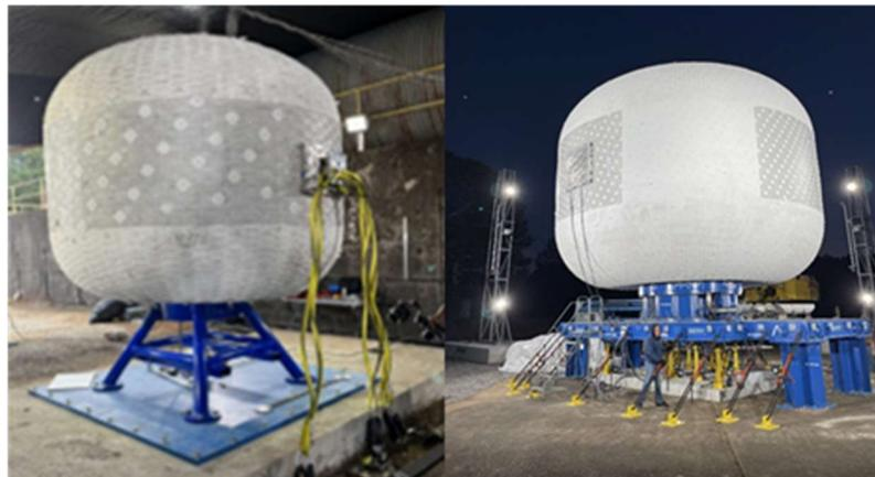
**Figure 1. LIFE 10 Subscale Module with One Blanking Plate and LIFE 285 Module with Two Blanking Plates 180 Degree Apart.**
