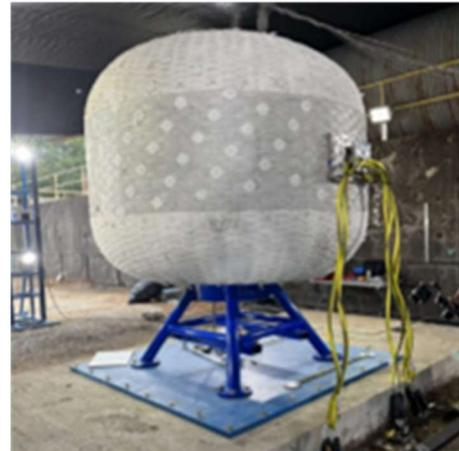
**Figure 6. Subscale Burst Test w/Blanking Plate.**
