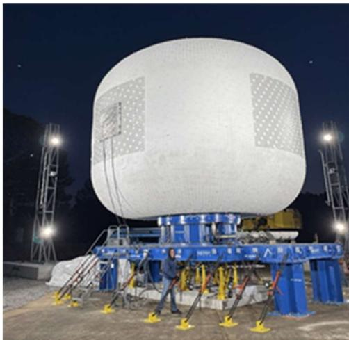
**Figure 7. LIFE 285 Ultimate Burst Pressure Test Unit #1.**
