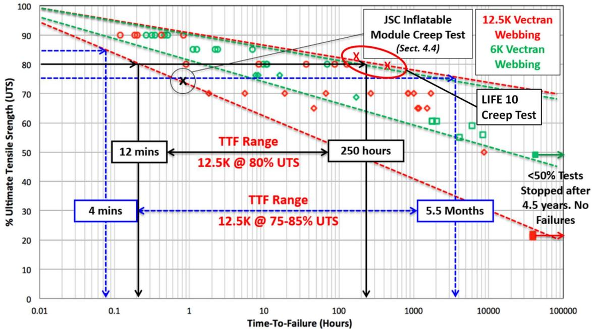
Figure 9. LIFE 10 Creep Test Results Plotted with Past Creep Results.
