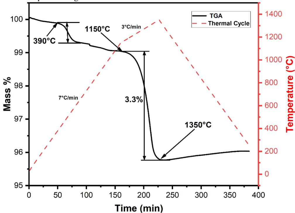
Figure 2. TGA of ore particle till 1350°C.
