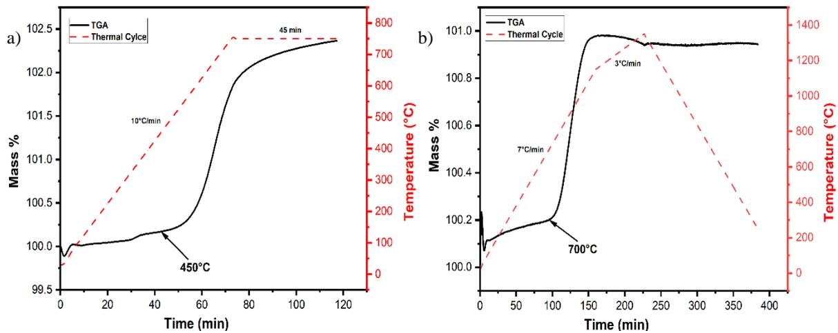
Figure 4. TGA results of ore particle a) Oxidation at 750°C b) second cycle of decomposition at 1350°C.
