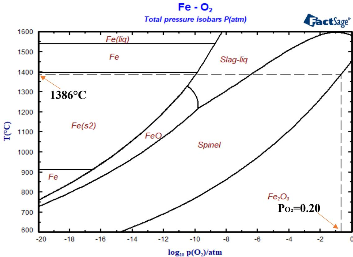
Figure 1. Fe-O<sub>2</sub> phase diagram calculated using FactSage.
