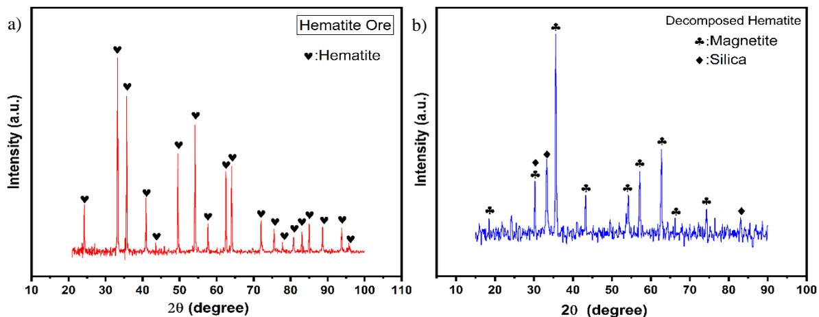
Figure 3. XRD pattern of a) Ore particle b) decomposed sample at 1350°C.
