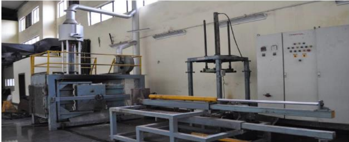
Fig. 1: Pilot coke oven in R&D unit, Vijayanagar Works, Karnataka
