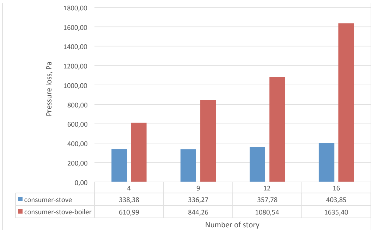
Figure 5. Schedule of pressure loss at the different number of stories in buildings taking into account design experience
