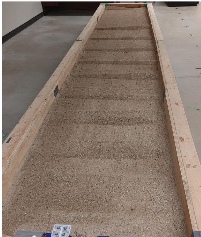
Figure 2: Sand Box used for this paper. The ridges that are shown in this image were small approximately 10 cm mounds that were created on the sand surface to represent an uneven surface and were added to induce wheel slippage. The positions of these waves were randomized in the experiments.
