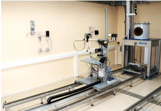
Fig.1. AT140 neutron calibration facility
