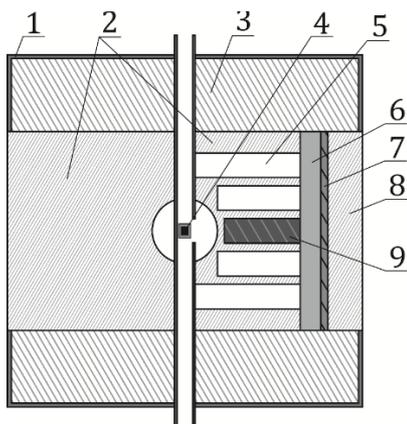
Fig.2. Monte-Carlo model of container-collimator with thermal neutrons geometry: 1 – aluminum casing; 2 – insert for thermal-neutron geometry; 3 – container-collimator; 4 –  $^{238}\text{PuBe}$  fast-neutron source (IBN-8-6); 5 – air channels; 6 – lead; 7 – target; 8 – polyethylene; 9 – tungsten.
