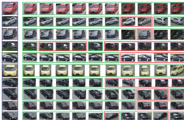
Fig. 3. Top-10 of the search results. The blue box indicates query images, the green boxes are correct hits, and the red boxes are incorrect hits.
