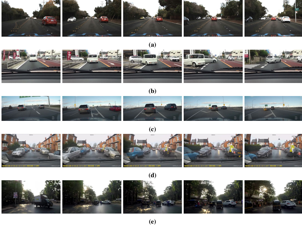
FIGURE 8: Sample Safety-Critical Episodes: (a). overtaking event in front of the car; (b). occlusion while turning left; (c). abrupt lane change on the highway; (d). pedestrian suddenly appearing from between two parked cars; and (e). (relatively) crowded and chaotic inner city traffic.
