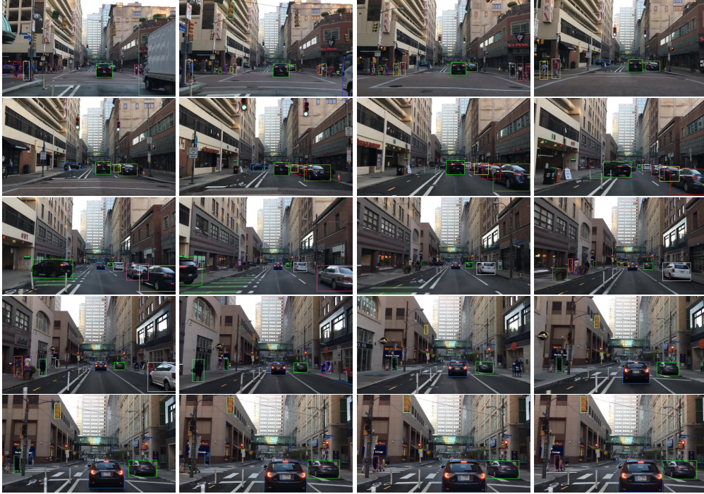
FIGURE B.17: Tracking results for the complete scene of the occlusion example (Fig 11; Section 4.1.2) involving tracking of cars, pedestrians, and traffic lights
