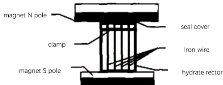
Fig.12 Magnetic field hydration reactor schematic
