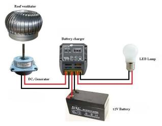
2. Install DC generator in the air ventilation ball and generator in the ball close to the axis. Put the gear in the proportion 1:4 to the air ventilation ball axis and rotor axis of the electric generator to allow the movement of electric generator axis while the wind blows the ventilation balls.
