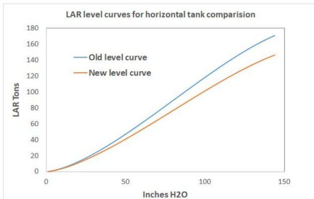
Figure#2 In this figure we can see the overestimation for the liquid contained in the tank where the difference% in weight was up to 14% approaching tank levels greater than 130 " of level water.
