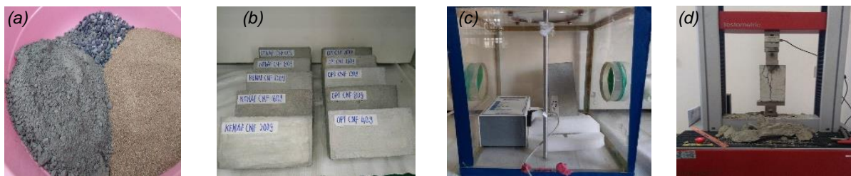
Figure 5: (a) Mixing of sand, stone, and cement (b) Fabricated composite brick (c) Radon gas measurement (d) Compression test
