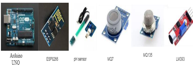
Fig: Devices and drives as sensors used in the IEE-PMCS module.
