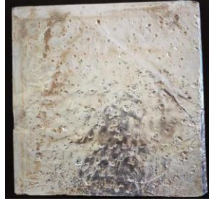
Fig. 2.2 Hail drop marks on the Hail-pad
