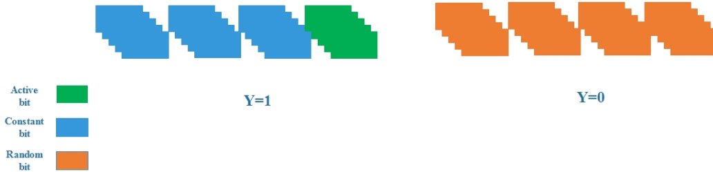
Figure 1: Dataset instances of our neural based Integral distinguisher: The multiset denoted by Y = 1 corresponds to integral properties of 1 active and 3 constant bits. Whereas, Y = 0 corresponds to the random multi-set in which no specific integral property is chosen.
