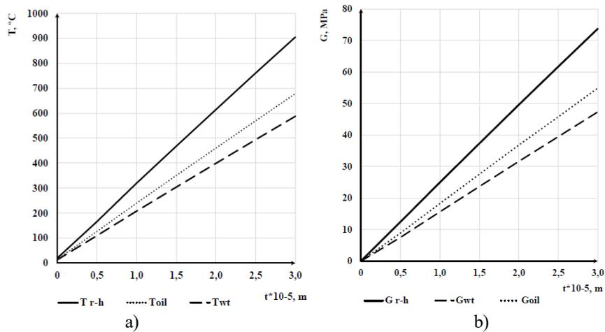
**Figure 4.** Contact temperatures (a) and residual stresses (b) when grinding CBN with wheels of structure No. 40 when cooling with air (using a Ranque-Hillsch tube), when cooling with oil and water-based coolant. Modes  $V_{cr} = 30 \text{ m/s}$ ;  $V_{det} = 0.166 \text{ m/s}$ ;  $S = 0.002 \text{ m/v}$  (LO250/160 C10 100% (Nz25))
