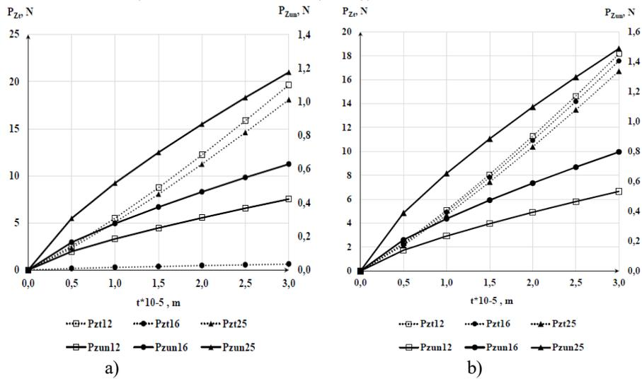
**Fig. 2.** The values of the unit and total cutting forces  $P_z$  during grinding with CBN circles of structure No. 6 - a) and structure No. 40 - b). Modes :  $V_w = 30$  m/s;  $V_{sp} = 0.166$  m/s;  $S = 0.002$  m / v. (LO250/160 C10 100% (Nz25))
