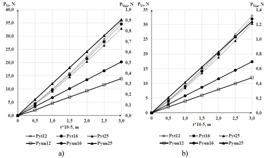
**Fig. 1:** The values of the unit and total cutting forces  $P_y$  during grinding with CBN circles of structure No. 6 - a) and structure No. 40 - b). Modes  $V_w = 30$  m/s;  $V_{sp} = 0.166$  m/s;  $S = 0.002$  m / rev (LO250/160 C10 100% (Nz25))
