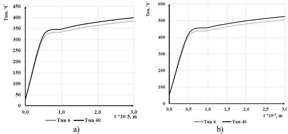
**Fig. 3.** Unit temperatures of grain cutting during grinding by circles. (LO250/160 C10 100% (Nz25)) of structure No 6 and No 40. Modes  $V_w = 30$  m/s;  $V_{sp} = 0.166$  m/s;  $S = 0.002$  m / v
