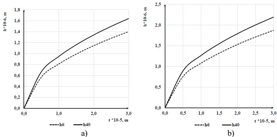
**Fig. 5.** The magnitude of the deepening of grain into material I when grinding CBN with wheels (LO250/160 100% (Nz25)) of structure No. 6 and structure No. 40. Modes  $V_w = 30 \text{ m/s}$ ;  $V_{sp} = 0.166 \text{ m/s}$ ;  $S = 0.002 \text{ m / rev}$ . Grain a)  $N_z = 12$ ; b)  $N_z = 25$
