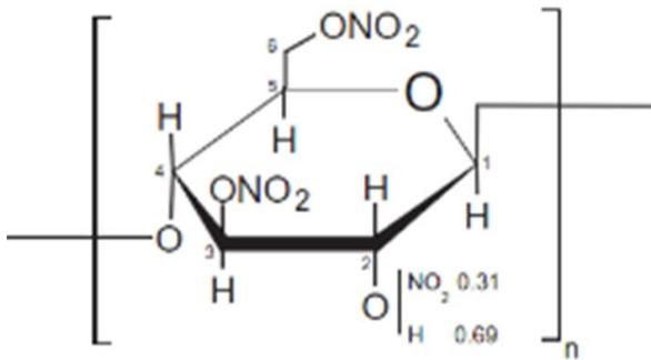
Fig. 4: Chemical structure of a nitrocellulose with a nitrogen content of 12.2% and degree of substitution, DS of 2.3 [15].
