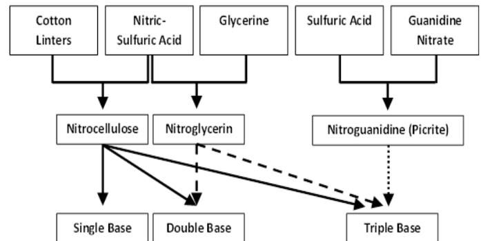
Fig. 5: Nitrocellulose Based Propellants
