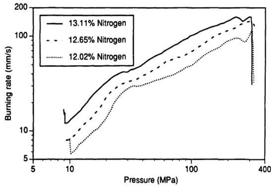
Fig. 3: Burn Rate Curves for Grains with Zero Perforations and Various Nitrogen Levels [13]
