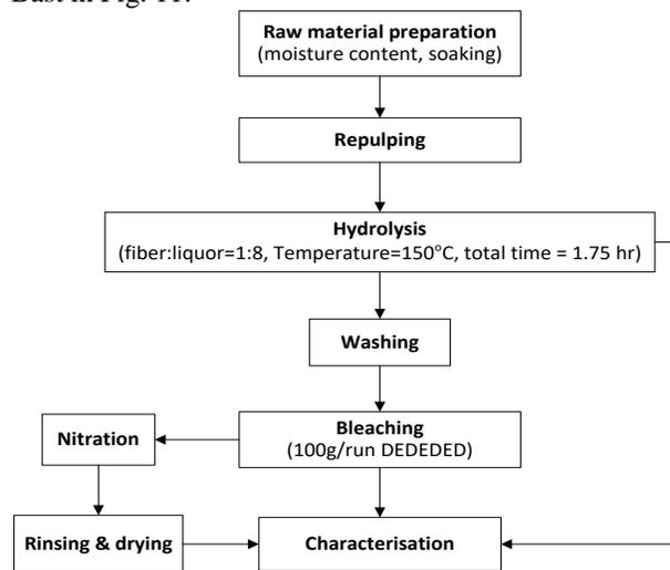
Fig.9: Overall nitrocellulose process flow for EFB
