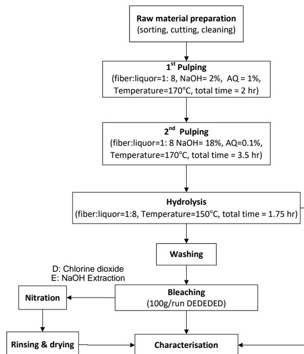
Fig.10: Overall nitrocellulose process flow for Rhizophora
