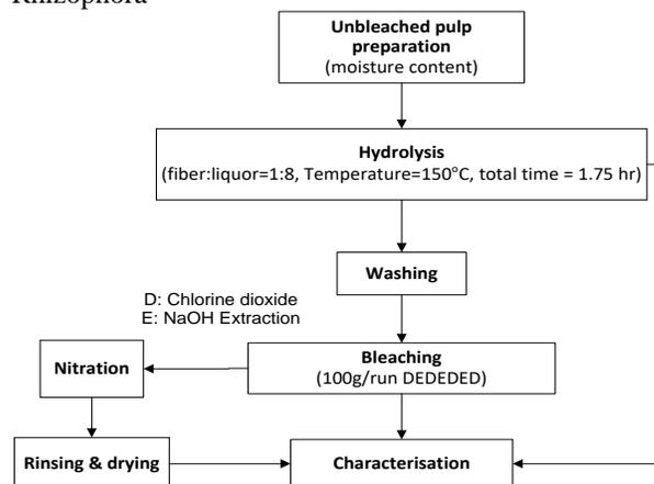
Fig.11: Overall nitrocellulose process flow for Kenaf Bast
