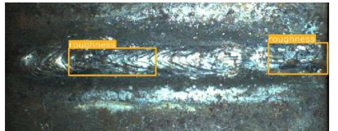
Fig. 10. Testing defect detection model on real weld sample.
