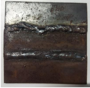
Fig. 1. Real weld sample with two weld beads
