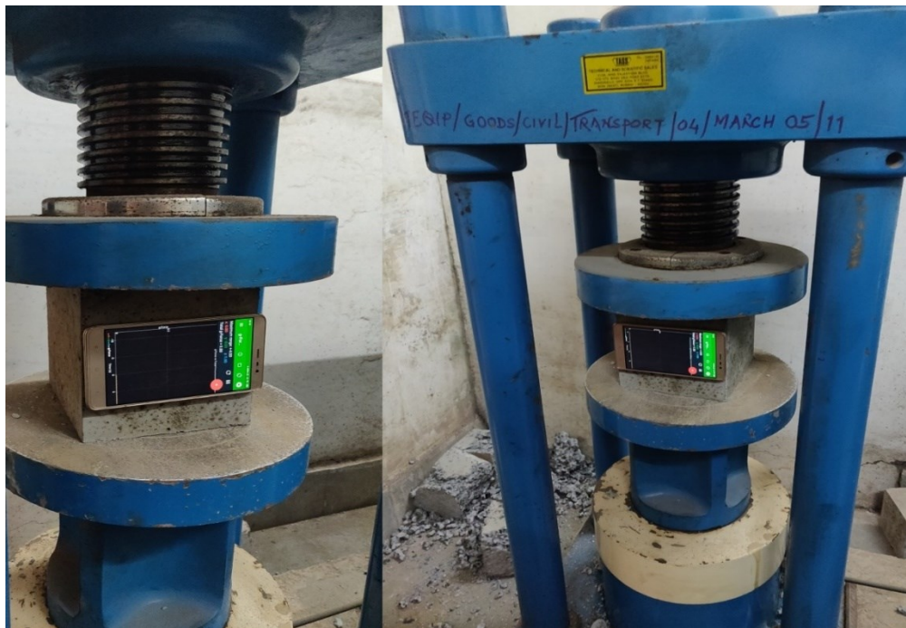
Figure 3. Testing of concrete cubes in which smart phone used as sensor for SHM
