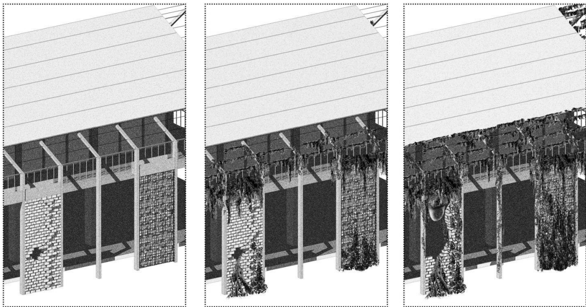
Fig 4. Mortar as bio-receptive element and Brick protrusion to control biological colonization (Aswin Senthil 2021) as part of Ecotone: The Sentient Ruins Studio, CEPT University, Tutored by Prof. Sonal Mithal
