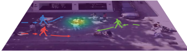
Fig. 1. GA-GAN uses the trajectory heat map to highlight gathering areas, and combines the the agent interaction algorithm to predict a reasonable trajectory.
