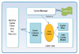
Fig 1. The Architecture of Web Cache System
