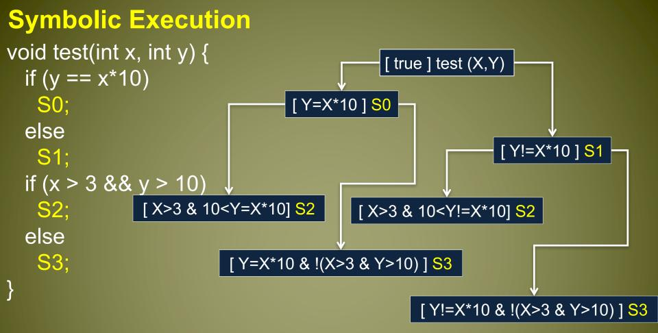
Test(1,10) reaches S0,S3 Test(0,1) reaches S1,S3 Test(4,11) reaches S1,S2
